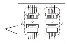
Following the labels (A to A & B to B) to plug the connectors.
